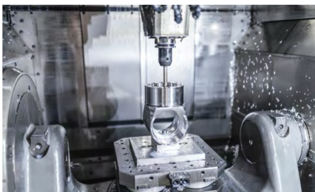
Producing a complex component for the aerospace industry on the C 22 U.
