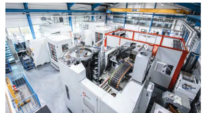
TVB uses the two C 22 U machines (in the background) exclusively for machining graphite. The robot loads the C 32 U (front right) with aluminium and brass components.
