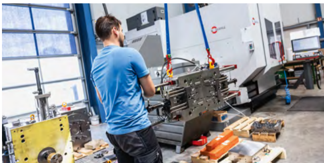
The multi-cavity mould, which S & S Werkzeugbau manufactured for Gardena, weighs several 100 kg.
